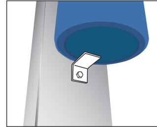
3. If you plan on holding a large cylinder and the base is not supported, it is advisable to use a piece of angle iron, wood block or shelf bracket to support the bottom of the cylinder. This will also make it easier to lock the clamp in place.
