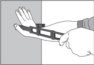
2. After fastening the SUPER QUICK FIST clamp, stretch the strap by putting one hand on the base and use the other to pull in a perpendicular direction several times on the strap.
